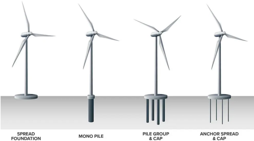
Different onshore wind turbine foundation types
